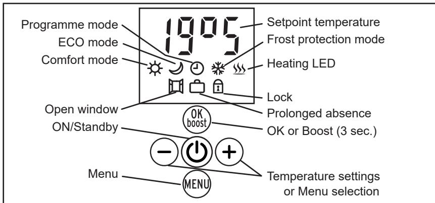
*The icon and the value being adjusted flash. Flashing stops when the setting is validated by pressing **OK-boost**, or after 30 seconds of inaction (any modification to the setting is then cancelled).*
