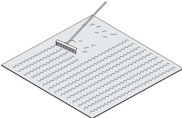
EN Even out and flatten the surface area with a rake.
