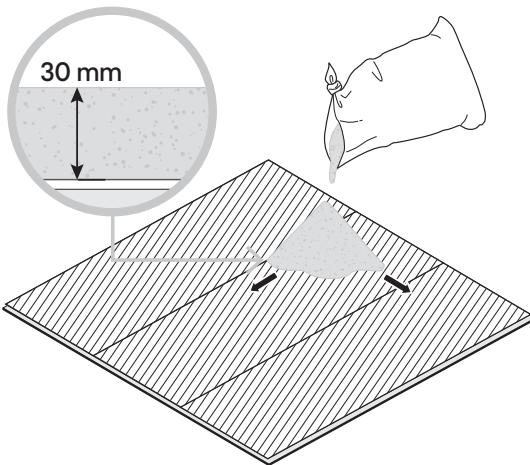
EN Lay sand to a depth of at least 30 mm.
