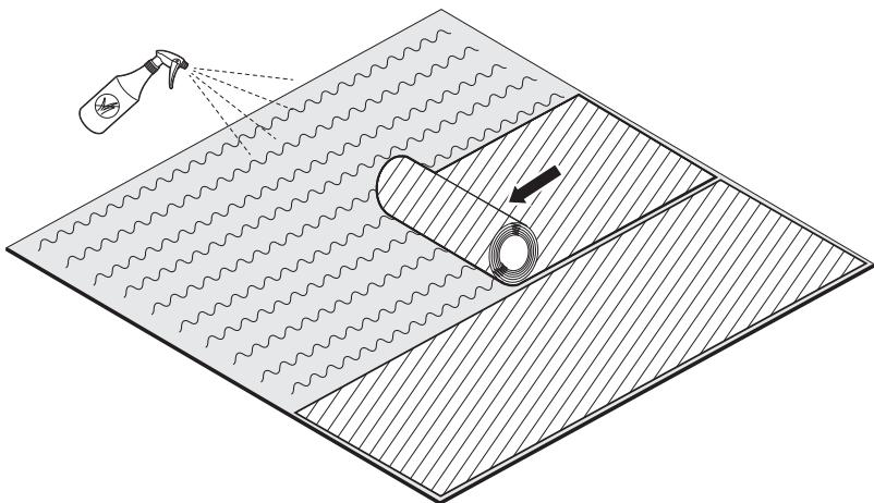
EN Spray weed killer then lay geotextile liner.
