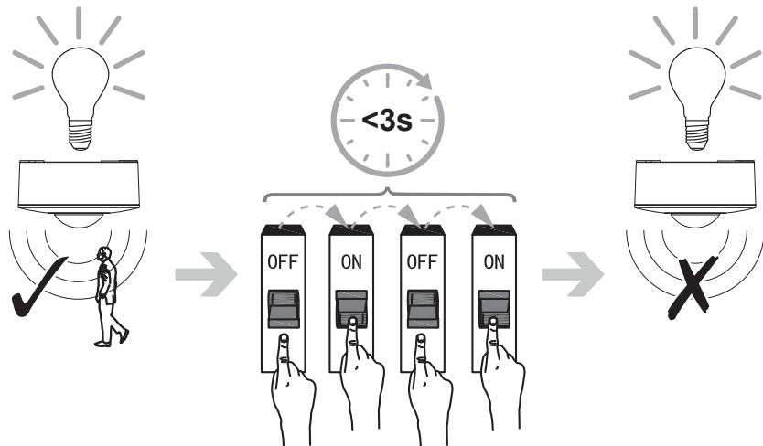
**EN** Deactivate motion sensor and keep light on
